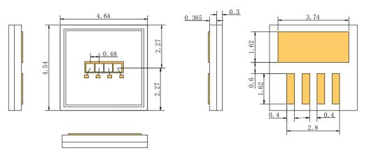
VD-0940P–050W –10–3A0 (Channel array 1x8, substrate AIN, Package 1x8)
