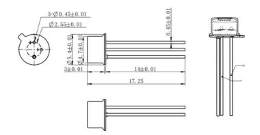
VD-0940P–050W –1N–3A0 (Channel array 1x4, substrate AIN, Package 1x4)
